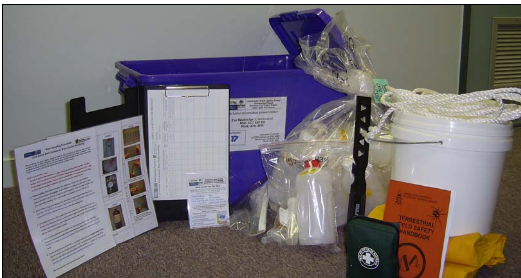
Figure 2 Volunteer Field Sample Box including clipboard with instruction sheet and sample record sheet, fridge magnet, water quality sample kits (containers, filters, syringes), bucket and rope, stirrer, first aid kit/manual and rain coats.
